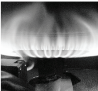
Proper burner flame pattern
