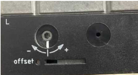
Detailed view of offset adjustment screw.
